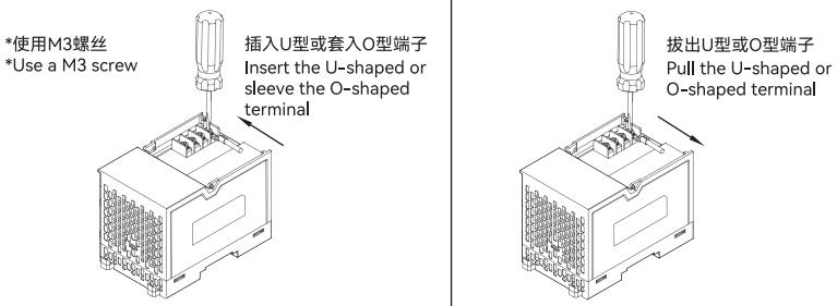
EN During connecting, use a small cross screwdriver to loosen the wiring screw, insert the U-shaped or sleeve the O-shaped terminal, and then tighten the screw. Gently tug the cable after pulling out the screwdriver. If the cable is secured firmly, then the connection is finished. The reverse is the procedure for unplugging the cable.
