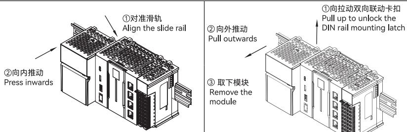
EN During mounting, align the groove of the power module to that of the controller, and then press it inwards until their lower parts click together. During dismounting, pull the power module outwards until it is detached from the controller, and then directly remove the module.
