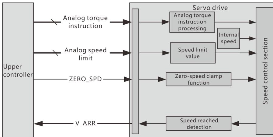
Figure 6.3 Block diagram of torque control mode
