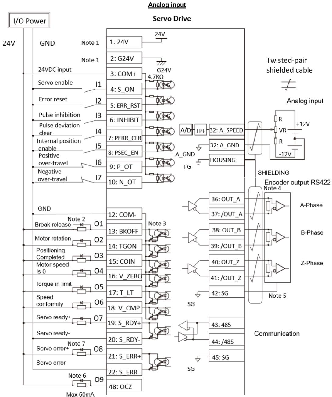
Note 1: Control power output (24V, G24V) can be used as I/O power (COM+, COM-). But the maximum output current is 150mA, and when driving the output such as relay and brake, please use external independent power.
