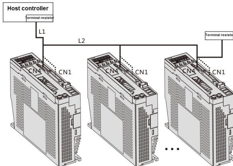
L1=5m (max): cables between upper controller and servo drive should be less than 5m.
