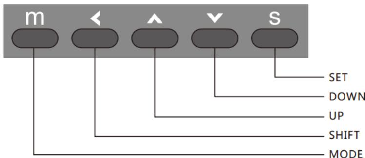
MODE button (m): switch level of parameters.
