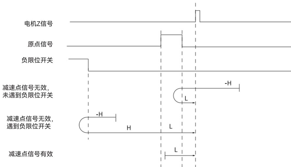
Figure 5-53 Homing Mode 11 Trajectory and Signal Status
